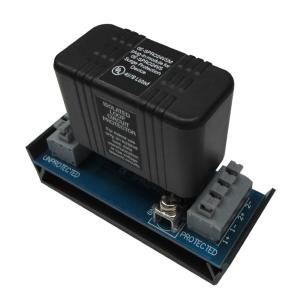
The OE-SPRO24VS surge protector protects up to two 24VDC or VAC, 4-20mA intrusion and fire alarm circuits and panels, including Signaling Line Circuit (SLC), Initiating Device Circuit (IDC) and Notification Appliance Circuit (NAC) loops. It consists of a snap track, base and field-replaceable plug-in module. It is designed for indoor use only and should be located in a telecom closet or listed enclosure. For field-replaceable plug-in module, order OE-SPRO24VSM.
